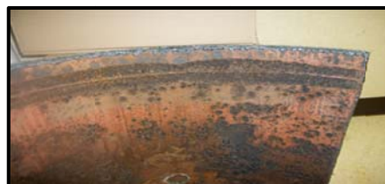
24" pipeline corrosion failure prior to application of SuperCorr ®
